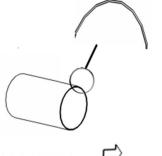
Press, with the thickest end first, the Snoot carefully over the fitting....
