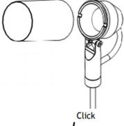
Press, with the thickest end first, the Snoot carefully over the fitting....
