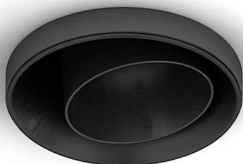
Exact, well-defined light from a flexible downlight that blends in with any surface. For indoor use. Roblon fibre optic technology. Recessed and adjustable. Low-glare. Mounting Ø22 mm. Rotates 360°. Tilts 10°. Beam angle 54°. For display, surface, object, area and accent lighting. For rooms, walls, ceilings, shelves, showcases, niches and many other applications.
