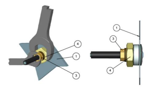
Assemble the fitting, pos 3, and the nut, pos 4, lightly by hand. Hold the fitting by means of a 14 mm wrench while tightening the nut by means of a 24 mm wrench.
