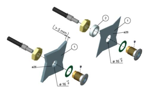
Guide the fibre through the hole and fasten ti in the fitting by means of the set screw. Around the hole an area of  $\emptyset 26$  mm must be completely plane. If this is not the case, joint with silicone. The space washer, pos 2, is only to be used when the wall, pos 1, is more the 5
