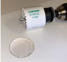
Drill Ø51 hull
