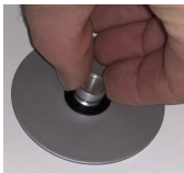
Press in the new reflector
