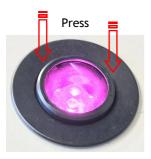
Place the filter in the holder and press the holder onto the lens
