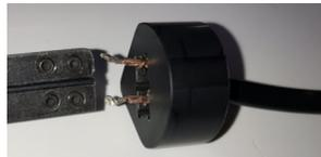
Connect the wires through holes in the end bracket.
