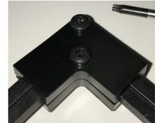
Place the rails in 90°. Mount the two wires, place the bottom fitting and top, screw it together with two screws.
