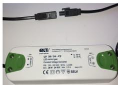
Place the light source on the track, connect the driver before turning on main power.
