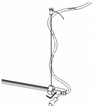
Mount electrical wire trough the End cap.
