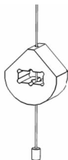
Lead the wire up through the Track support from the bottom until it reaches top and the square hole is not blocked.
