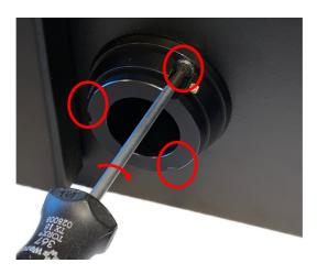
4. Screw the front part on to the light generator.
