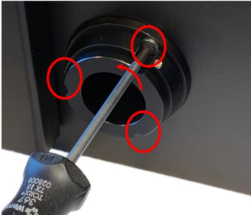
1. Unscrew the front part from the light generator. Do the work in a dry clean environment.
