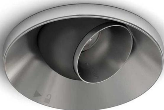
Exact, well-defined light from a flexible downlight that blends in with any surface. For indoor use. Roblon fibre optic technology. Recessed and adjustable. Low-glare. Mounting Ø64 mm. Rotates 360°. Tilts 35°. Beam angle 54°. For display, surface, object, area and accent lighting. For rooms, walls, ceilings, shelves, showcases, niches and many other applications. This product is available in a bronze version on request.
