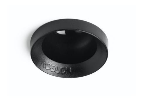
Precise, powerful light from a tiny, simple downlight. For indoor use. Roblon fibre optic technology. High light efficiency. Recessed and fixed. Low-glare. Mounting Ø25 mm. Beam angle 54°. For display, surface, object, area and accent lighting. For showcases, niches, shelves, ceilings and many other applications.
